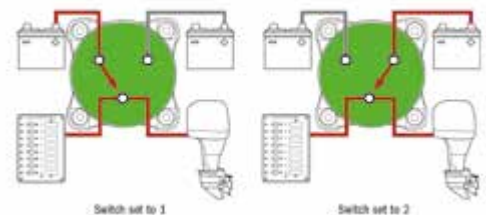
Switches isolated battery banks to all loads
