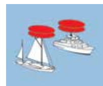
In addition to starboard, port and stern lights: 2 All-round red in vertical line
